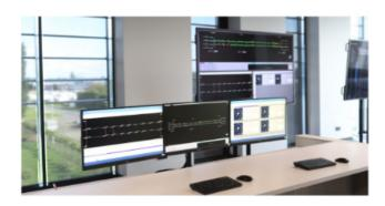
At one of the largest railroad stations in Poland, RCC Warszawa Główna Towarowa- Warszawa Jelonki, our system enables management of 150 switch point machines and 164 signals. Kombud has integrated the remote control centre with computer, relay and mechanical systems operating at adjacent stations.
